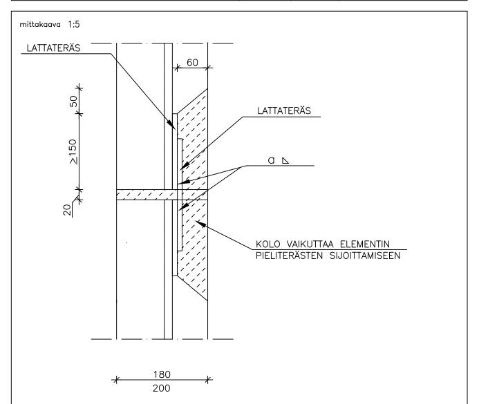
VETOTERÄKSEN SIJAINTITOLERANSSI VAIKUTTAA LIITOKSEN VETOKAPASITEETTIIN
