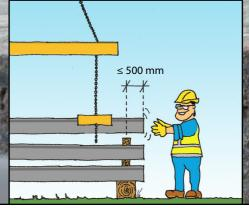
ALWAYS STORE THE HOLLOW-CORE SLABS ON AN EVEN, STABLE SURFACE AND STACK THEM ON BOTTOM AND INTERMEDIATE SUPPORT TIMBERS.
