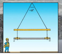
FOLLOW THE MANUFACTURER'S INSTRUCTIONS WHEN SELECTING LIFTING POINTS. THE ANGLE BETWEEN THE LEGS OF THE LIFTING CHAINS MUST BE LESS THAN 60 DEGREES.
