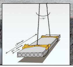
A SLAB THAT IS SHORTER THAN THREE METERS CAN BE LIFTED WITH LONG LIFTING CHAINS WITHOUT A SPREADER BEAM.
