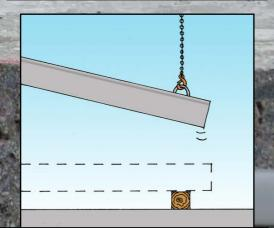
SLABS THAT ARE MEANT TO BE INSTALLED IN A TILTED POSITION SHOULD ALWAYS BE LIFTED BY USING LIFTING LOOPS OR ANCHORS.
