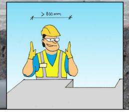
CLAMPS CAN ONLY BE USED TO LIFT A NOTCHED SLAB IF THE INTACT PART OF THE SLAB IS AT LEAST 800MM LONG.
