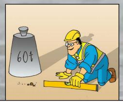
PREPARE A ROAD THAT IS SUFFICIENTLY WIDE, EVEN AND STABLE. CHECK THE GROUND BEARING CAPACITY UNDER THE CRANE OUTRIGGER.
