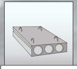
USE LIFTING LOOPS TO LIFT SMALL SLABS.
