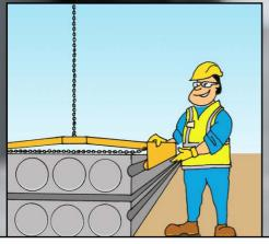
PLACE THE PROTRUDING LIP OF THE CLAMP CAREFULLY INTO THE GROOVE OF THE SLAB.
