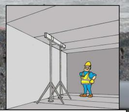
ASSEMBLE THE TEMPORARY SUPPORTS FOR THE WORK PHASE ACCORDING TO THE PLANS, PRIOR TO THE INSTALLATION OF THE SLABS.
