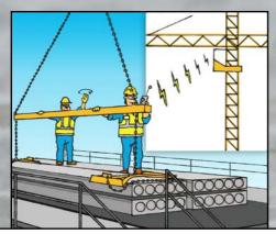
THE HOLLOW-CORE SLABS WILL BE INSTALLED BY USING A SPREADER BEAM AND LIFTING CLAMPS. MAINTAIN EYE OR RADIO CONTACT WITH THE CRANE OPERATOR.
