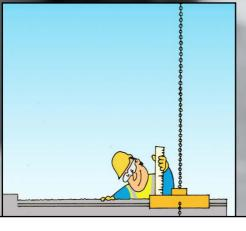
MAKE SURE THAT THE LIFTING GROOVES OF BATHROOM SLABS ARE IN ORDER.
