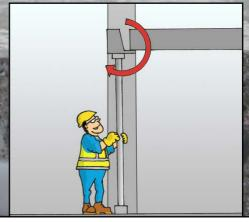
PREVENT THE TILTING OVER OF A BEAM BY PROVIDING SUPPORT, ACCORDING TO THE PLANS, CLOSE TO THE END OF THE BEAM.
