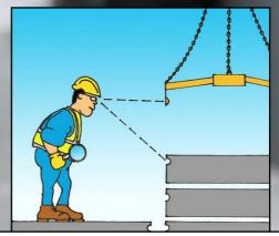
INSPECT THE LIFTING GROOVE AND ENSURE THAT THE PROTRUDING LIP AT THE BOTTOM OF THE CLAMP FITS INTO IT. DO NOT LIFT A DAMAGED SLAB.
