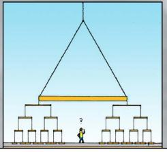
VERIFY THE AMOUNT AND TYPE OF LIFTING CLAMPS THAT ARE REQUIRED FOR HEAVY SLABS.
