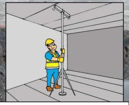
LEVEL OUT DIFFERENCES IN THE SLAB CAMBER, ACCORDING TO THE PLANS, BY USING SUPPORTS, ADJUSTER BOLTS OR INSTALLATION SHIMS.
