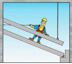
USE SUPPORT IN THE FORM OF WELDED STOPPERS OR BY WEDGING A TILTED SLAB INTO PLACE WHEN POSITIONING.
