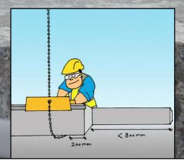
IF THE NARROWED END OF THE SLAB IS SHORT, ATTACH THE CLAMPS 200MM FROM THE EDGE OF THE NARROWED PART OF THE SLAB.
