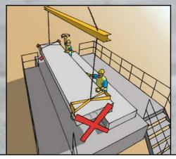
WATCH OUT FOR ANY SWINGING MOVEMENT OF THE SLAB AND POSITION YOURSELF SAFELY ON THE LONG SIDE OF THE SLAB.
